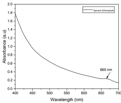
**Figure 8** Absorption Spectrum of Chlorophyll dye solution
