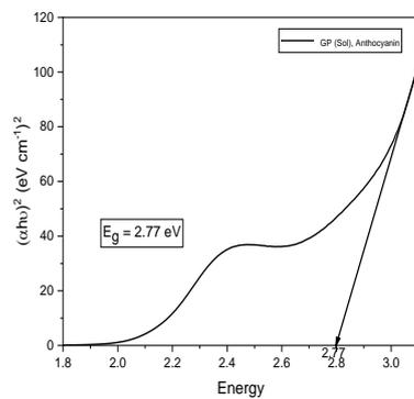
**Figure 11** Energy band gap of Anthocyanin dye solution
