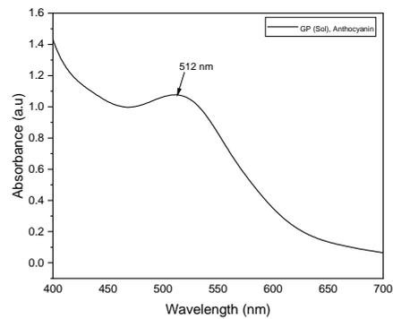
**Figure 9** Absorption Spectrum of Anthocyanin dye solution
