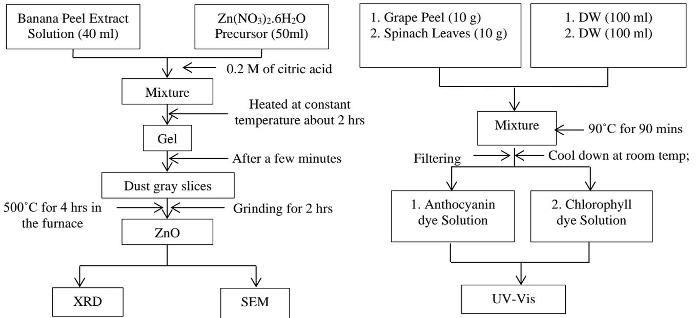
**Figure 1** Flow-chart for green synthesis of Oxide Nanoparticles
