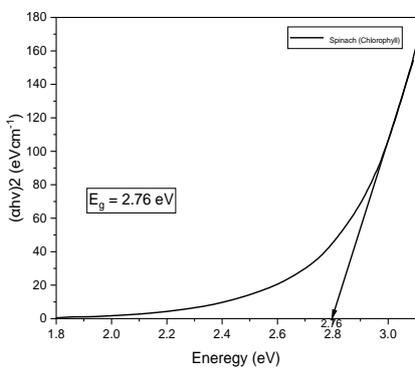
**Figure 10** Energy band gap of Chlorophyll dye solution
