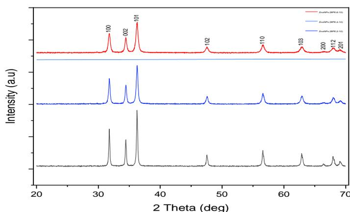
**Figure 4** XRD patterns of ZnONPs (2:10, 4:10, 6:10)
