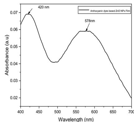
**Figure 13** Absorption spectrum of Anthocyanin dye based ZnONPs
