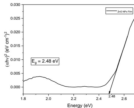
**Figure 7** Energy band gap of ZnONPs film
